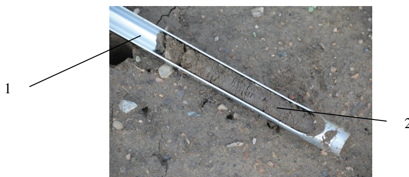
Fig. 1. Manual probe: 1 – sampling tube; 2 – extracted core
