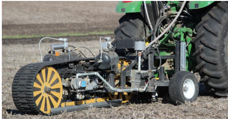
Fig. 2. Autoprobe automatic soil sampling device pulled by ordinary tractor
